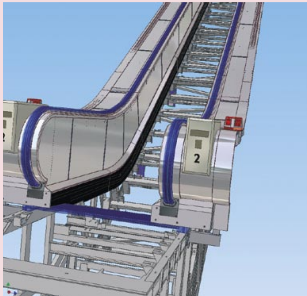
Figure 4. Inventor model showing the construction of an escalator truss with partially completed passenger-side balustrade in place
